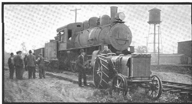
Pulling a Locomotive and One Car With a Bryan Light Steam Tractor at Peru, Indiana
